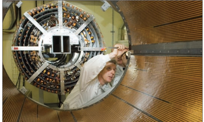
Checking clearances before the ATLAS Semiconductor Tracker barrel, in the background, is inserted into the Transition Radiation Tracker.
